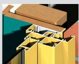
Standard 30mm jamb with built-in nailing fin/ weather bar into brick veneer wall illustrated above.
