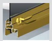
Awning sash inlay can be operated with cam handles as shown above or manual chain winders as shown on next illustration.
