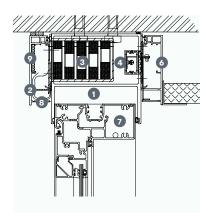
Standard configuration shows the AWS Trickle Vent mounted within sub-head. Optional angle bracket to accommodate suspended ceiling tile.
