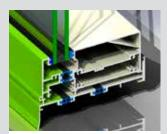
Sub-sill designed to support heavy double glazed frames and maintain the thermal break – dual colour option. We offer FrontGLAZE™ in both internal or external glazing.
