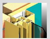
Alternative bold 44mm wide jamb with built-in nailing fin/weather bar illustrated above. Both 30mm and 40mm frames will accept height adjustable galvanised building-in lugs.
