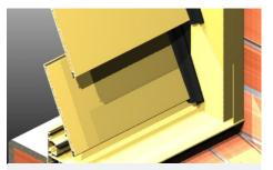
We offer 102mm and 152mm aluminium blades. Each blade is fitted with a co-extruded Santoprene weather seal where the blade meets blade. Blades can be coloured to match main frame if required.
