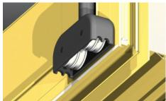
Bottom rollers are more reliable for residential projects as top hung panels can run into problems if the head lintel sags.
