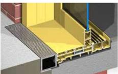
The above illustration shows the completely flat sill design feature. It features a four track XXXF flat sill with recessed sump on the outside and Centor S1 roller screen on the inside.
