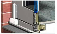
This illustrations shows the 316 stainless steel roller cowling - designed for coastal applications. Bottom rollers allow us to have heavy door panels as the weight is supported by the sill as well as the option of highlights being fitted above.
