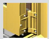
Heavy duty hinges: Custom light zinc die-cast or heavy duty extruded hinge nests into the frame and door stile. This significantly increases the hinge strength which is important when doors are large and/or heavy.
