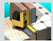
Fitting custom parliament hinges to French doors (80mm frame) allows panels to be opened back 180° to the wall lining when positioned correctly in building.
