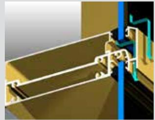
Concealed drainage designed to shed water more efficiently and improve aesthetics without runs of visible holes along the face. Very high water performance greater than 600 Pa.
