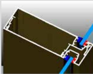
Expansion mullion shown above with extra weather leg behind glazing pocket, providing high water resistance. We can use silicone wet top on the outside in lieu of the captive wedge.
