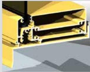
Sub-sill, sub-head and sub-jamb available. The sub-sill has additional support leg under the glass, designed to carry weight of heavy glass unit and prevent frame dishing.
