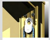
One sheet of glass counterbalances the weight of the other via a heavy duty ball bearing pulley (rated to 300kg) and high strength cord (rated to 300kg).
