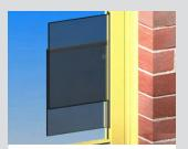
Two panes of glass slide silently past each other within aluminium guides which fit neatly into the perimeter frame.
