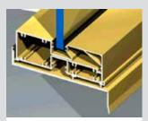
All 620 framing is designed to accept thick glass up to 15.38mm. The central support leg in sub-sill shown above helps support the weight of heavy glass units and prevent frame dishing.
