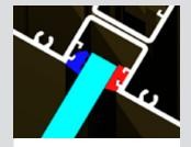
Frame designed to accept captive wedge or spacer. We can use Silicone wet top on the outside in lieu of the captive wedge.
