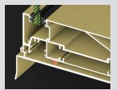
Sub-sills have central support leg, designed to support the weight of heavy glass panels and prevent sill dishing.
