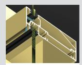
Concealed drainage in transom allows water to escape via face of the system.
