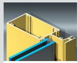
Series 626 Structural offers 15mm of structural glazed adhesion around all four sides of IGUs.
