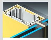
Variety of mullion options including interlocking mullion with stiffener option available to allow mullion withstand higher wind load.
