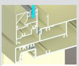
On externally beaded sashes the standard bead configuration is square however splayed beads are available.
