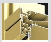
Series 665 sashes are fabricated as a hook hinge design, single or double glazed.
