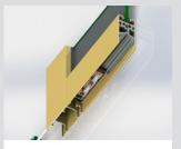
Bottom rolling doors run on heavy duty double or quad bogey wheel carriages
