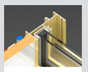
The sash is concealed below the reveal and maintains the same sightlines as the fixed lights for greatly enhanced thermal performance.
