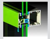
Designed to accept 24mm IGUs. Glazing pocket offers the required 12mm glass bite on IGUs. A variety of pocket closer extrusions are available should thinner glass be required.
