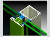
We offer both snap-together and expansion mullions. We recommend expansion mullions on long runs of framing (over 6m).
