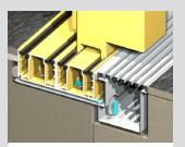
Can accept sliding door panels in a variety of commercial applications. This fully recessed sill is completely flat and still keeps water out. Complies with AS1428.
