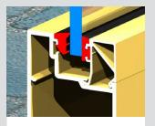
We offer security glazing as shown above. Captive co-extruded glazing wedge on the outside. We can use silicone wet top on the outside in lieu of the captive wedge.
