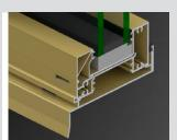
Wide 50mm glazing pocket accomodates IGUs up to 44mm thick, ideal for applications where high performance glazing packs are used to improve energy efficiency or accoustic performance.
