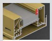
Pocket reducer makes it possible to reduce the glazing pocket dimension so thiner IGUs can be accomodated
