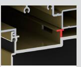
Stiffening rail in sill helps to support heavy panels and ensure smooth operation and long-term durability.
