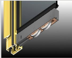
Vantage wheels have been designed to fit snugly into the door bottom rail. Nothing slides as smooth as a Vantage sliding door. As shown above, double or quad bogey wheels are used on heavy doors.
