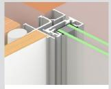
Thermal performance is achieved by reducing the exposed internal boundary and the ability to transfer energy through the aluminium frame.
