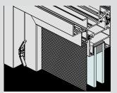
Fly screens can be easily fitted with custom nylon clips located on the jambs/mullions.
