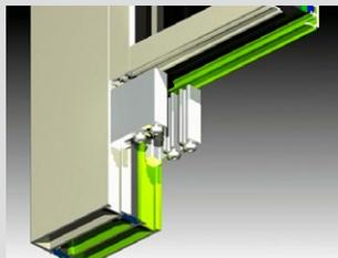
Commercial doors are only as good as the joinery system. Series 852 doors have custom extruded aluminium spigots and backing plates that ensure the joint between the stiles and rails remains tight.
