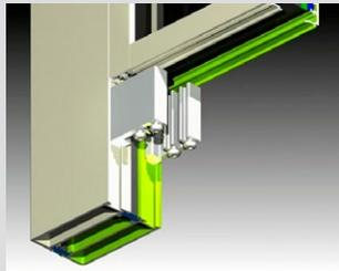
Commercial doors are only as good as the joinery system. Series 852 doors have custom extruded aluminium spigots and backing plates that ensure the joint between the stiles and rails remain tight.
