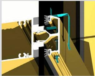
Concealed drainage holes are designed to shed water more efficiently.
